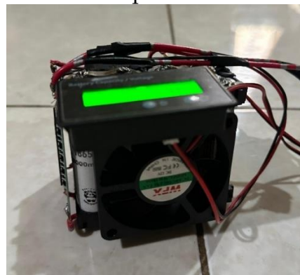
Pic. 5 Battery with fan cooling
