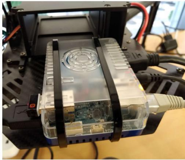
Figure 4: Experimental embedded setup: Odroid-XU4 board installed on DJI Matrice 100 drone.
